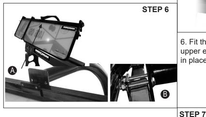
6. Fit the shield assembly into the bracket on the upper end of the support column (A) and secure it in place using the supplied hardware (B).
