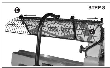
8. Push in towards the installed end (A) to fit the second pin in the other mounting hole (B).
