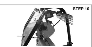
Note: Always keep the shield latched in place using the hooks, during operation.
