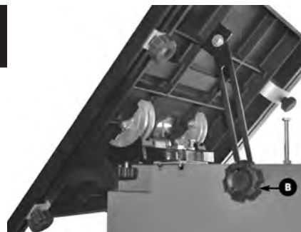
FIGURE 24: TABLE TILT ADJUSTMENT
