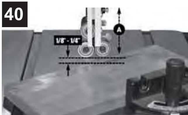
FIGURE 41: BLADE GUARD ADJUSTMENT
