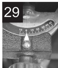
FIGURES 29 and 30: ANGLE POINTER ADJUSTMENT
