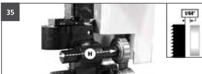
FIGURE 35: BLADE GUIDE ADJUSTMENT
