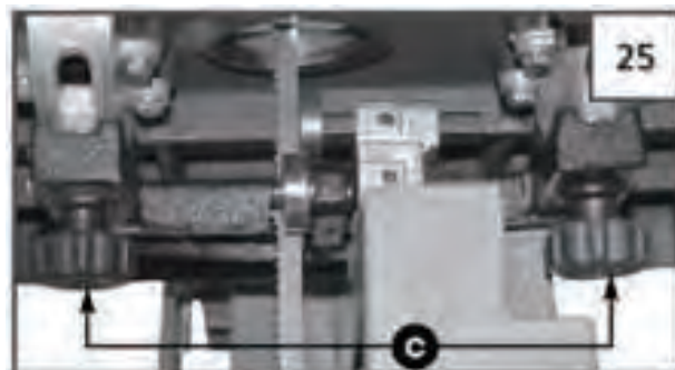
FIGURE 25: TABLE TILT ADJUSTMENT
