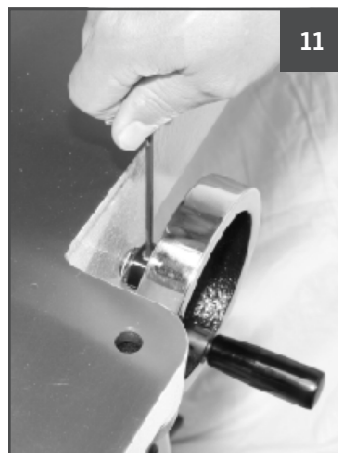
FIGURES 10 & 11: INSTALLING TABLE HEIGHT ADJUSTMENT HANDWHEELS
