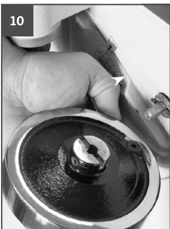
FIGURES 10 & 11: INSTALLING TABLE HEIGHT ADJUSTMENT HANDWHEELS
