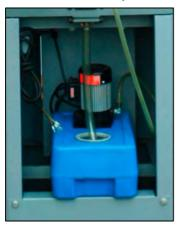
Found within the machine stand, the coolant pump is a self contained system that includes a tank, pump motor, filters and hoses.
