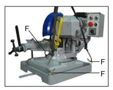
Prepare the machine unit for hoisting
