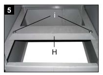
Attach the coolant tank platform.
