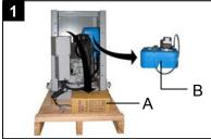
Take out the accessories (A) and the coolant tank (B) from inside of the stand and set aside for later use.
