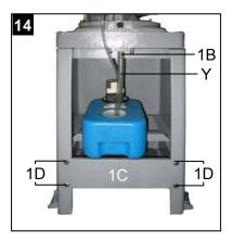
Attach the rear plate to the back of the stand.
