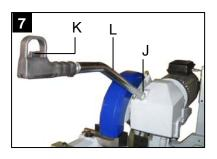
Attach the control handle to the head assembly.
