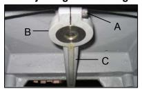
The lock lever may require adjustment when the lever is limited by the machine base and it fail to adequately secure the miter angle for machine head. If there is insufficient brakeage of the lock lever:
