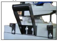
A Device that support longer sized material. The roller assists stock moving through the vise.
