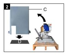
Lift off the stand (C) and place into the intended working location (D).
