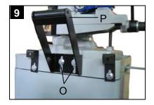
Attach the support roller to the left side of the base.
