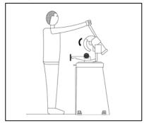
The operator should stand in front of the machine using a single hand to grip the control handle.
