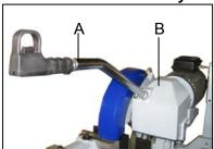
The section of the machine composed motor, gear transfer system, disc or blade, and control handle.
