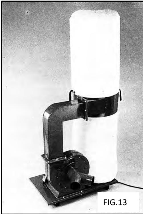
The dust collector is now ready to be placed into serviced. Before connecting to a power source, be sure the power source is properly grounded and is of proper voltage amperage FIG.13.
