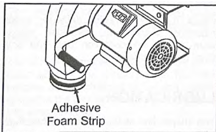
Figure-4 Installing adhesive foam strip
