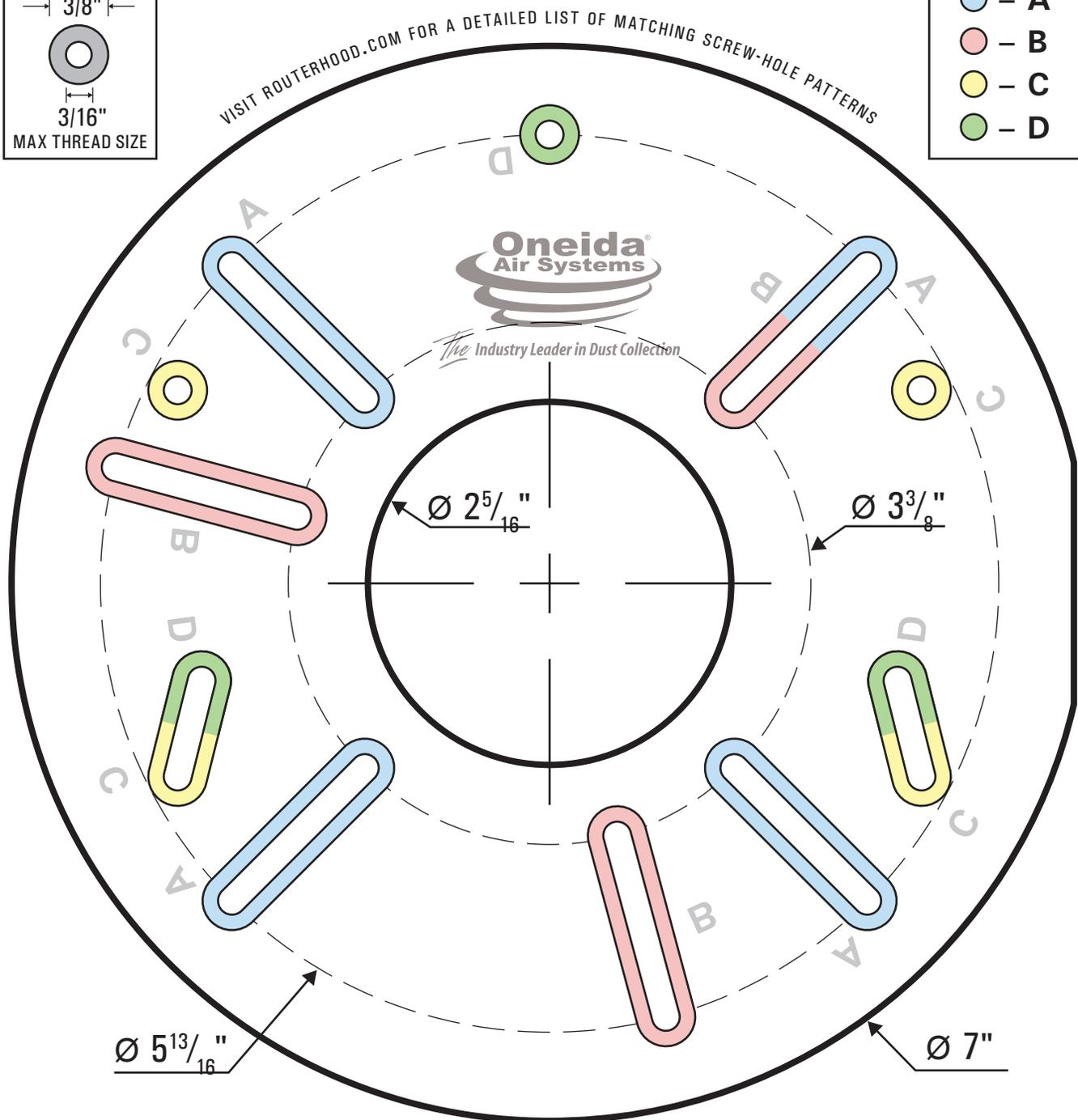
In addition to confirming screw hole compatibility, ensure that your router base has a center hole diameter of at least  $2\frac{3}{8}$ ". A router base with a smaller center hole will not work with the Dust-Free Router Hood.
