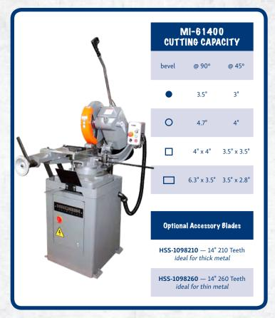
For tight tolerances and clean finishes when cutting metal, a cold cut saw is your best bet. This heavy-duty 14" model from Magnum Industrial delivers precise cuts in a variety of ferrous metal cutting applications—angle stock, pipes, extrusions and more. It features variable-speed cutting with a digital speed display, high-capacity coolant tank, and quick-clamping vise that makes loading and unloading more efficient.
