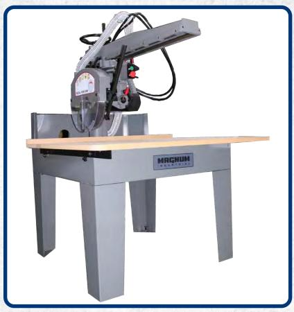
Designed for continuous-duty production shops, the MI-53400 Heavy-Duty 16" Radial Arm Saw features impressively sturdy castings and a rugged overall construction. It also comes with a variety of safety features including a blade brake, safety guard, riving knife, mag switch and motor return. The MI-53400 delivers accurate results in many applications — crosscuts, rips, mitre cuts, bevel cuts and more — and fine adjustments are easy to make.
