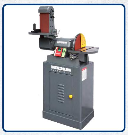
Magnum Industrial's heaviest belt and disc sander, this machine delivers 1,800 RPM and tons of torque — perfect for wood and metal sanding applications in professional production shops and schools. This sander is available with two different motors (see specs below) and features thick cast-iron tables, a cast-iron backing disc and an enclosed stand.
