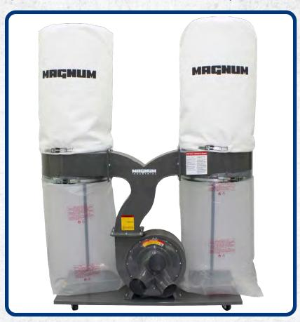
Delivering both power and capacity, the Magnum Industrial MI-11400 dust collector features two filter bags, two collection bags and an aluminum anti-spark impeller — driven by a fully enclosed 3 HP motor. This collector is designed to provide central dust collection for a medium-to-large production shop.
