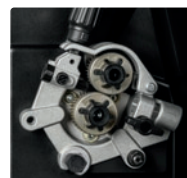
Heavy-duty aluminum two-drive-roll system
